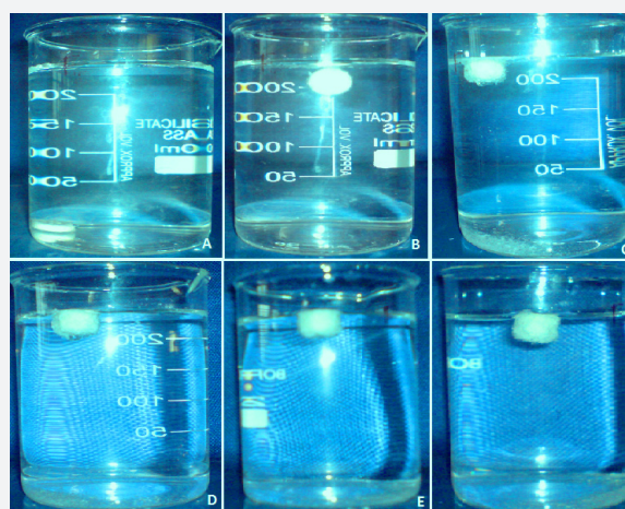
Figure 2. In vitro buoyancy test of Imatinib mesylate floating tablets in 0.1 N Hcl after 10 sec ( A ) 64 sec ( B ) 2 min ( C ) 4 hours ( D ) 8 hours ( E ) and 12 hours ( F ).
